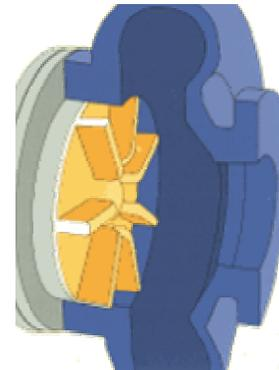
In operation, some of the fluid is drawn into the rotating impeller and discharged back into the casing through centrifugal action. Through fluid dynamics, the partial flow through the impeller imparts a centrifugal rotating motion to the entire fluid body within the casing. Large solids entering the casing are transported by the rotating fluid body from inlet to outlet without necessarily making contact with the impeller.
