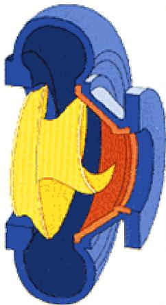
The screw centrifugal pump impeller is shaped like a tapered Archimedes screw. Originally developed for pumping live fish, the screw centrifugal pump has become popular for many solids handling applications, especially those where gentle handling is an important consideration.
