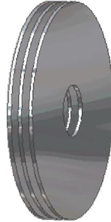
Slip, or the difference in speed between the disc and each layer, increases with distance from the impeller. The effectiveness of a disc impeller is related to the spacing of the discs and the viscosity of the fluid. Close disc spacing and higher viscosity produce better performance than low viscosities with wider disc spacing.
