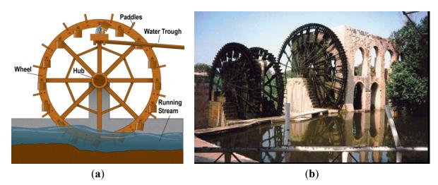
Figure 2. Waterwheel (Noria): (a) parts; and (b) in Hama on Orontes River in Syria (adapted from [27]).
