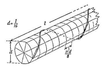
**Figure 9.** Design of the endless screw of Archimedes based on the description of Vitruvius (adapted from [44]).
