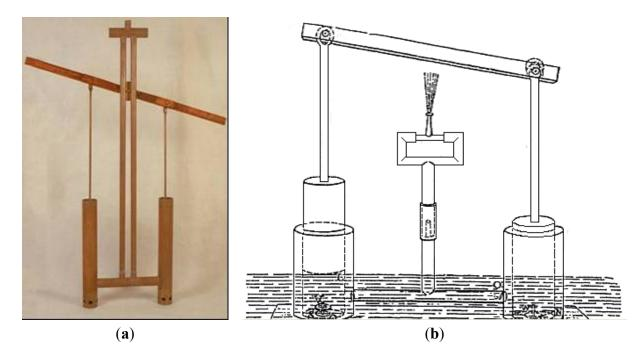
Figure 11. Ktesivius force pump as described by: (a) Philon; and (b) Heron with adjustable nozzle (adapted from [52] and [53] respectively).
