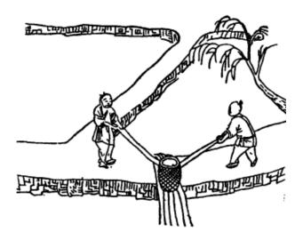
Figure 6. Schematic illustration of water lifting scenario with the Hùdǒu [40].
