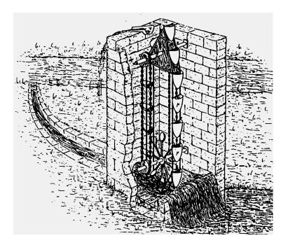
Figure 10. Philon's paddle-wheel driven bucket-chain (adapted from [48]).
