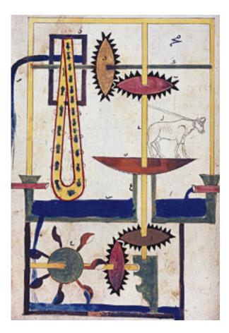
Figure 18. Al-Jazari's hydropowered saqiya chain pump device (adapted from [70]).
