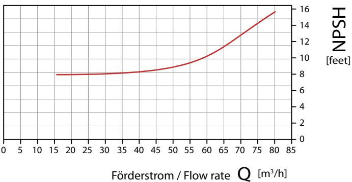
— 50 Hz - cycles | 2900 1/min - rpm - tr/min
