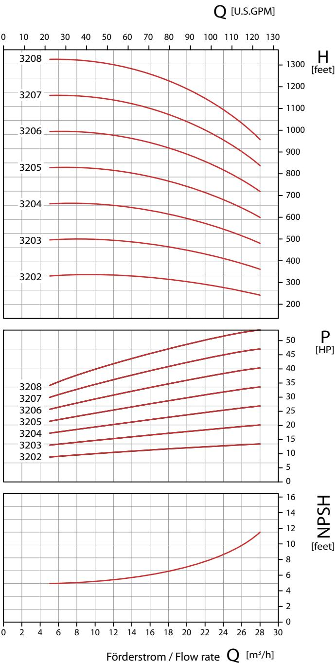
— 50 Hz - cycles | 2900 1/min - rpm - tr/min
