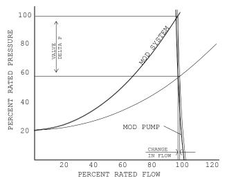
Fig. 2-3. Modified Curves: Discharge Throttling
