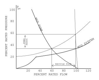
Fig. 2-5. Modified Curves: Recycle Control
