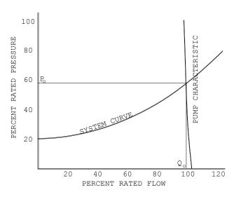
Fig. 2-2. Pump Characteristic and System Curve
