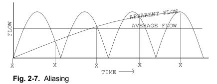
Flow measurements on the discharge of high pressure pumps should be avoided. This may not be possible if the pump has a recycle loop that returns, as it should, to the suction vessel. In that case remember that the flow sensor will experience not onlv hiah pressure but also a high level of
