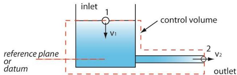
Here are some other examples of control volumes. The reference plane does not always have to be the lowest point. In pumping systems, the pump suction centerline is usually taken to determine the reference plane and all the elevations are taken with respect to the suction.
