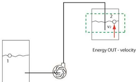
Energy (kinetic) OUT  $\frac{m v_2^2}{2}$
