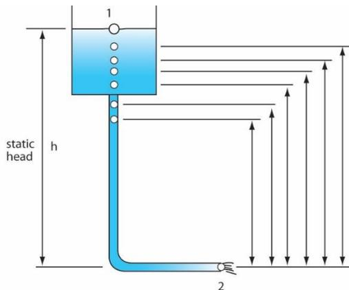
Point 1 is the highest point in the system. Let's assume that the level is remaining constant, the particles around point 1 will eventually make their way out of the system. The height of point 1 with respect to the outlet at point 2 is called the static head of point 1 or if we are connected to a pump or a turbine it would be called the suction static head.
