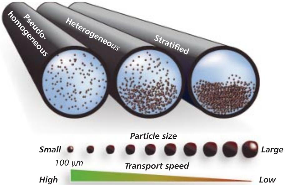
*A high transport speed and/or small particles means that all the particles are in suspension. The slurry behaves pseudohomogeneously.*
