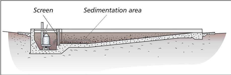
Smaller sumps with sloping walls create turbulence and high velocity in the sump, preventing the slurry from settling. Settling solids slide down into the zone directly under the pump inlet.
