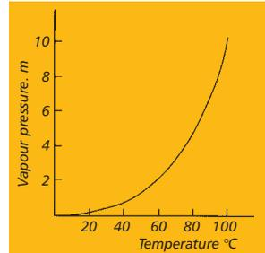
*Vapour pressure for water at different temperatures*
