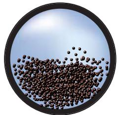
*Heterogeneous mixture, fully stratified*
