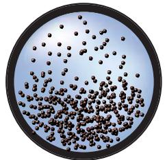
*Heterogeneous mixture, partly stratified*
