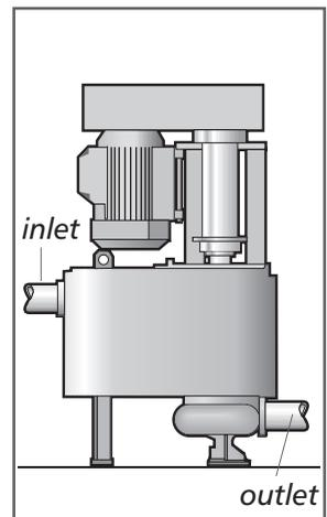
Cantilever/sump pumps are considered as *semi-dry installed*, as the hydraulic end is lowered into the slurry, but the drive unit and support structure are dry installed. Similarly to tank pumps there are no submerged bearings or shaft seals, but a long shaft overhang.
