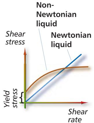
**In applications where the pumped slurry is viscous or non-settling, other methods of calculation are required instead of FLYPS or the manual calculations described in this book. Contact your Flygt support for advice.**
