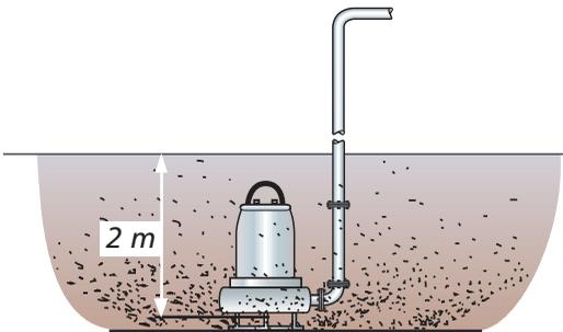
The value of  $NPSH_a$  must exceed the value specified for the pump,  $NPSH_{req}$
