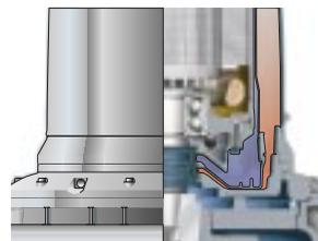
*Pump with internal cooling system*
