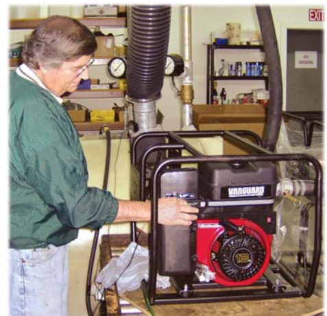
Bench Testing Riverside Pumps
