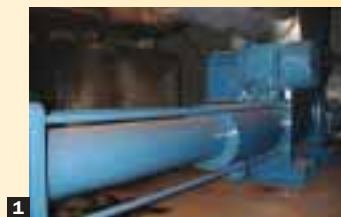
1 feeding of a GBB with silo outlet
