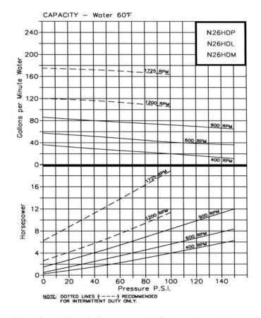
Note: Dotted lines (---) recommended for intermittent duty only due to accelerated wear at high speeds and pressures.
