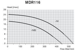
Based on water at 20°C, 50 Hz, 2800rpm
