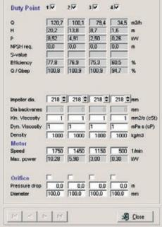
Example: CL 100-200 with 7.5 kW motor 50 Hz (8.6 kW at 60 Hz).
