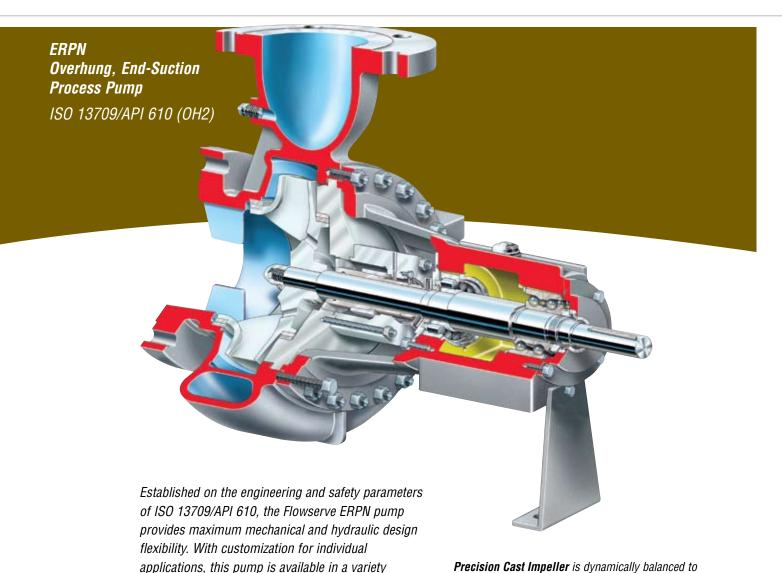
of optional configurations, including:Closed impeller with front and back wear rings for standard services
