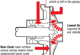
Lowest Overall required NPSH of any standard pump
