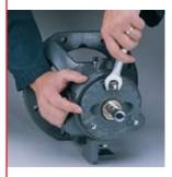
Move the bearing carrier clockwise the selected number of notches. Tighten the setscrews and check the impeller clearance with the feeler gauge.
