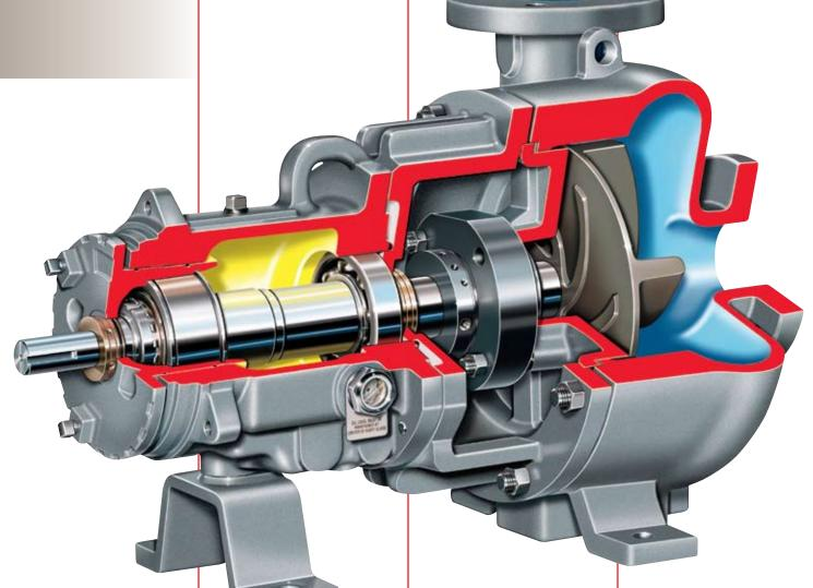
**Vortex Action** minimizes abrasive wear while maintaining solids integrity because only a fraction of the media contacts the impeller
