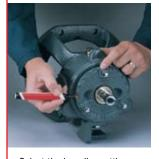
Select the impeller setting. Each notch on the carrier ring represents exactly 0.10 mm (0.004 in) of clearance. For an impeller setting of 0.5 mm (0.020 in) count five notches counterclockwise.
