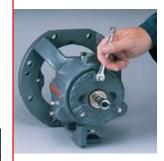
Simply loosen the setscrews. Using a wrench rotate the bearing carrier counterclockwise until the impeller lightly touches the rear cover plate.
