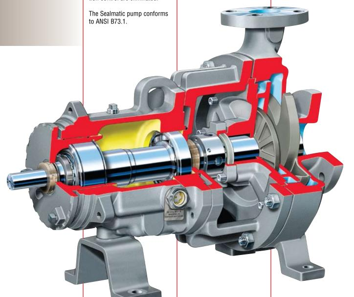
External Micrometer Impeller Adjustment accurately sets impeller clearance in 20 seconds, in the shop or the field
