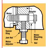
Unique C-Plus Precision Alignment System (Four Point) routinely delivers shaft alignments below 0.05 mm (0.002 in) in less than 30 minutes.
