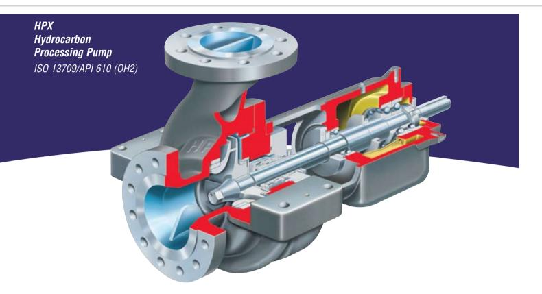
The HPX pump is the workhorse of the hydrocarbon processing industry, boasting unequaled versatility, reliability and safety. Designed to withstand the high pressures and temperatures often found in the oil and gas and hydrocarbon industries, the HPX is a horizontal end-suction pump with a top discharge, overhung, centerline-mounted configuration. It is fully compliant with ISO 13709/API 610 (OH2) latest edition design criteria and features an ISO 21049/API 682 compliant seal chamber.
