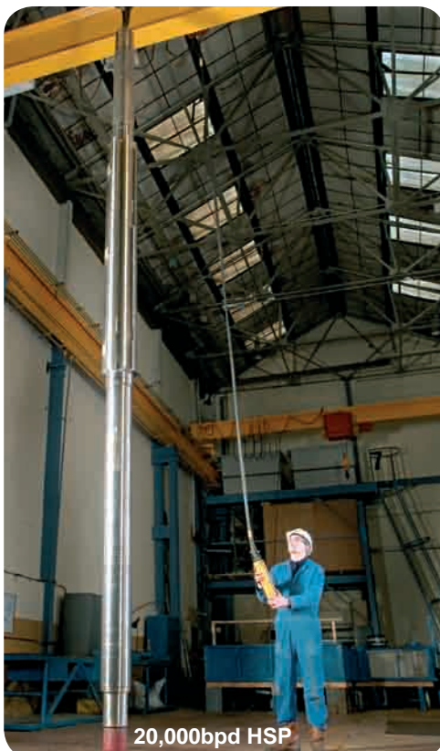
DOWNHOLE COMPLETION FOR WIRELINE CONVEYED HYDRAULIC DRIVE DOWNHOLE PUMP
