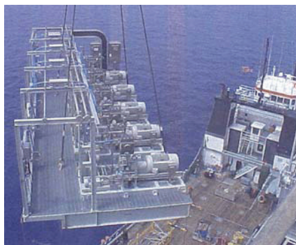
HDP 115 units for methanol duty Op. pressure 15,000 psi – 1035 bar Flow rate 1.5 gpm – 6 l/min
