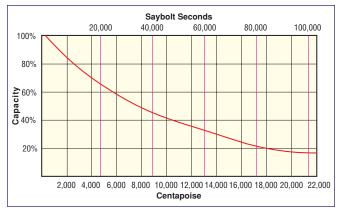
As you can see from the diagram above, as viscosities increase, the capacity of the pump decreases. Do not exceed 22,000 centapoise or 100,000 saybolt seconds on all 3/8" up to 3" pumps. Do not exceed 4,000 centapoise or 18,000 saybolt seconds on 1/4" models.
