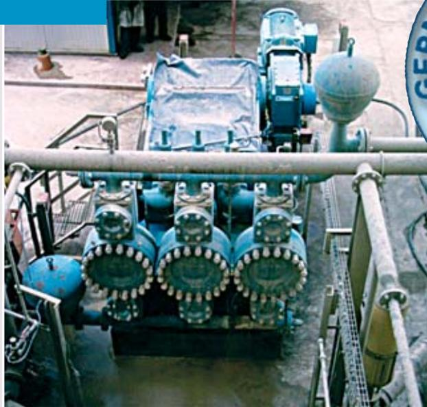
*Suction and discharge side pulsation dampeners on an ABEL HMT pump*
