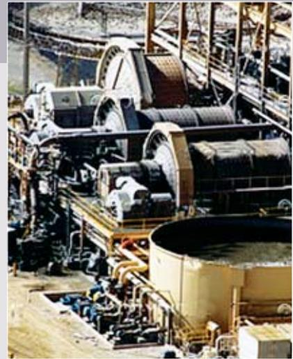
ABEL HM pumps are in operation at a lignite fired power plant in North America for the transfer of abrasive fly ash. Solids concentration is almost 75%. Similar pumps are transferring gold tailings in South America. Other interesting applications can be found in India (bauxite), Zambia (copper), Czech Republic (power), Norway (nickel), Brazil (magnetite) and many more countries, worldwide.
