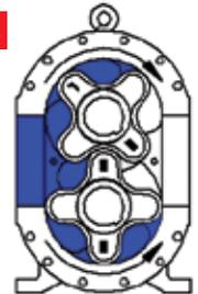
Fluid travels around interior of casing.
