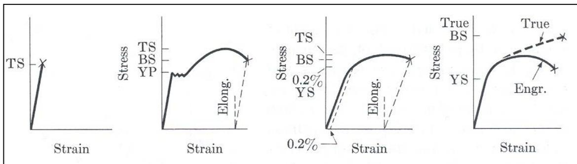
Figure 1. Definition of stress terms in a deformation test (reference *Elements of Material Science* by Van Vlack, Addison-Wesley Publishing Company, 2<sup>nd</sup> edition).
