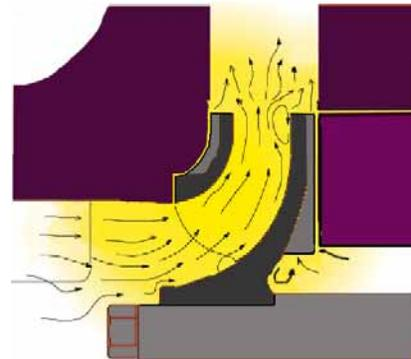
The disadvantage of pump-out vanes is that they consume power while controlling leakage and thrust. When new, a pump impeller equipped with pump-out vanes will likely have a lower efficiency than its wear ring counterpart. However, it will come close to maintaining its “as installed” efficiency throughout its operational life.
