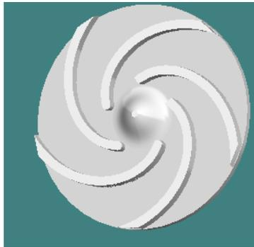
A semi-open impeller operates more efficiently than an enclosed impeller because of lower disc friction and tighter axial clearances. It has an advantage over an open impeller in that it can be adjusted axially to compensate for casing wear.
