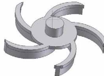
An open impeller typically operates at a higher efficiency than a shrouded impeller of the same specific speed. The largest contributor to efficiency loss in an enclosed radial impeller is disc friction caused by the front and back impeller shrouds turning in close proximity to the stationary casing walls. (See the [Sept 2004 newsletter](#) on efficiency). Removing the shrouds eliminates the disc friction.
