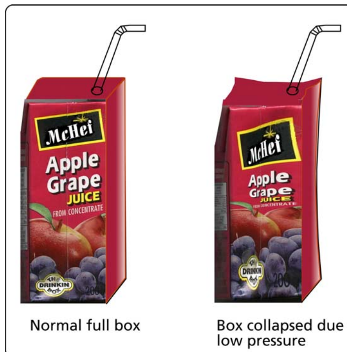
Figure 13 A full juice box at the same pressure as atmospheric pressure vs. a full juice box with the juice under low pressure and the box collapsed.
