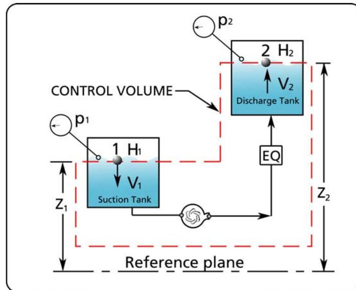
Figure 2 A general representation of a pumping system.
