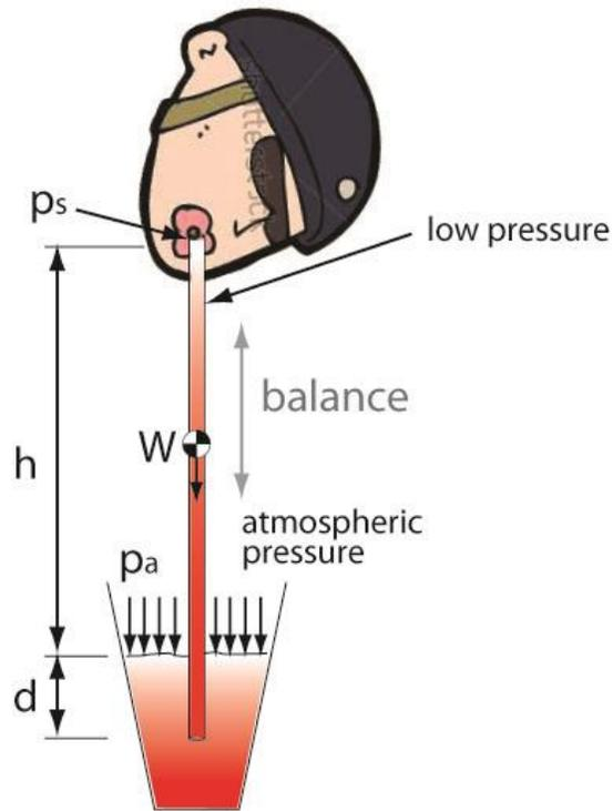
Figure 2. Using atmospheric pressure and suction to suspend water.
