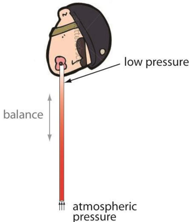
Figure 1. Using atmospheric pressure and suction to suspend water.
