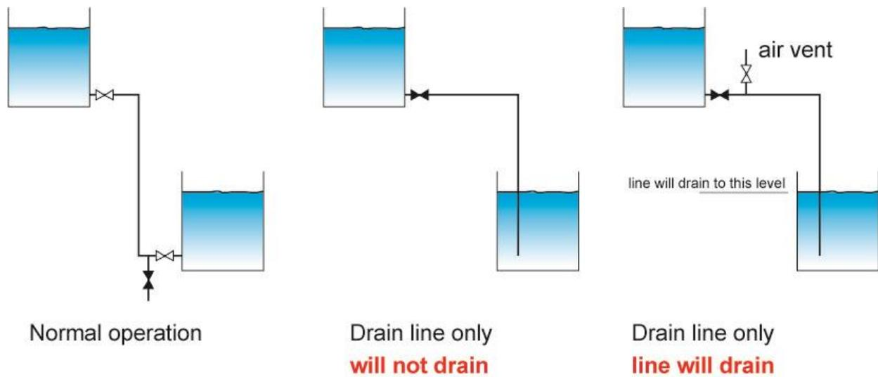
Figure 4. Air vent required to drain line.
